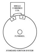
5. No Battery operated ignition allowed. Only a passive ignition system using R.P.M. as the single input parameter is allowed.
